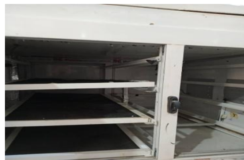
Figure 3: The interior view of solar drying system drying chamber
